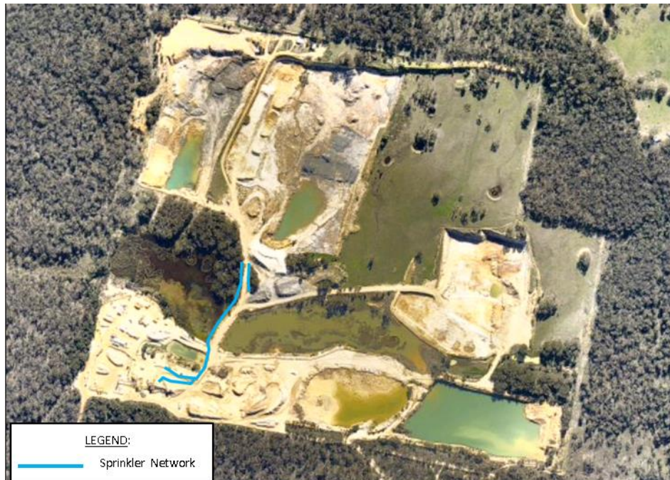
Figure 3 – Dust Suppression Sprinkler Location
