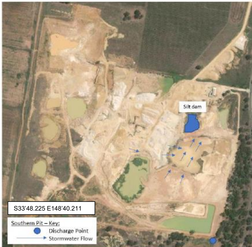
Figure 2: Site Surface Stormwater Directional Flows
