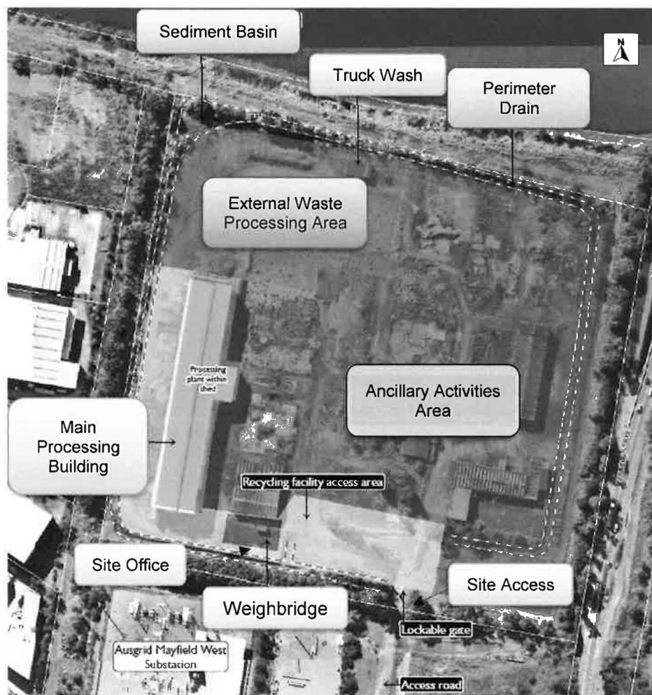
Figure 2: Existing Site Layout
